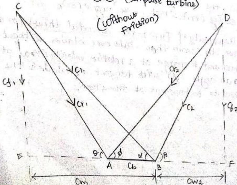
\* For solving problems on turbines, it is a common practise to combine two velocity diagrams on a common basis representing blade velocity ( $c_b$ ), when there is no friction.
