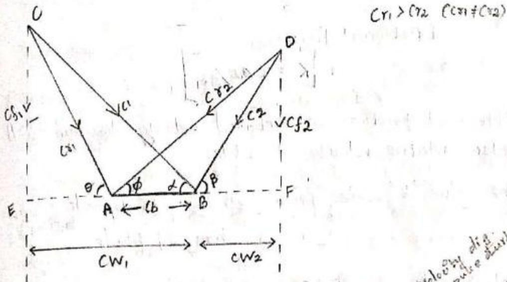
Velocity diagram for Reaction turbine:
