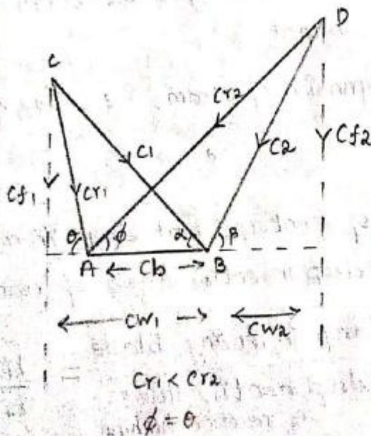
Velocity diag. for impulse turbine without friction
