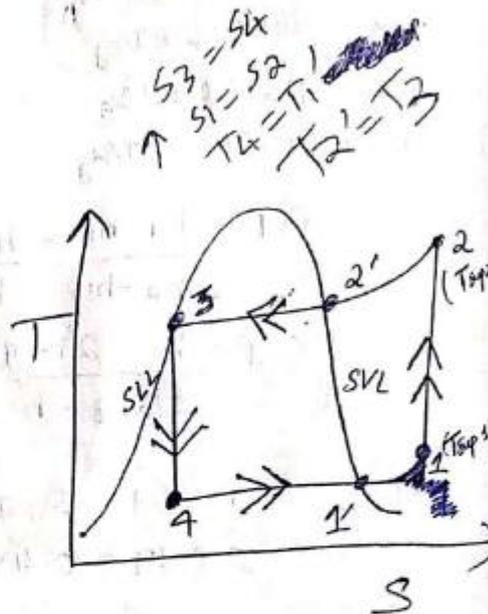
$$\text{COP} = \frac{h_1 - h_4}{h_2 - h_1}$$
