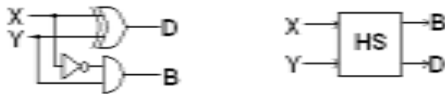
Fig 1.3 : The half-subtractor circuit and the symbol
